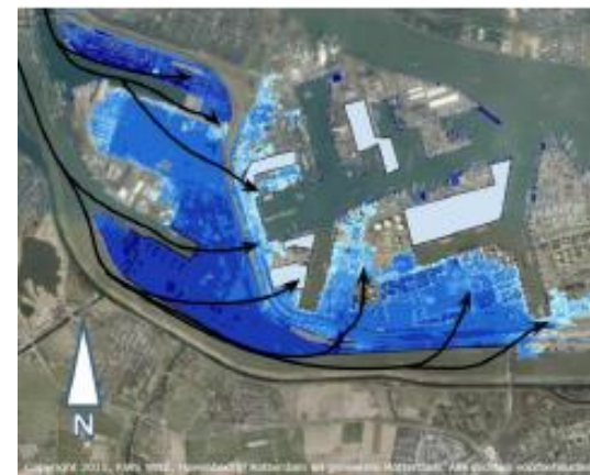
Figure 4-11 Flooding of zone 3 in detail (Event with a probability of 1/10,000 in 2050)
